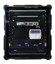
Totally autonomous and self-sustained, the system only requires 230V power feed, even if an onboard UPS will support operability during short period of time.
