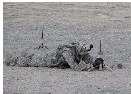
Fig. 2: Installation of an UGS.
