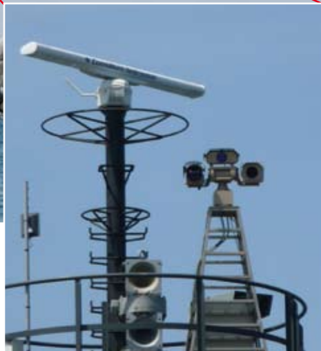
The HRC-S MS in the port of Ravenna is installed on a 14 meter high mast, located at the end of a 3 kilometer long pier.
