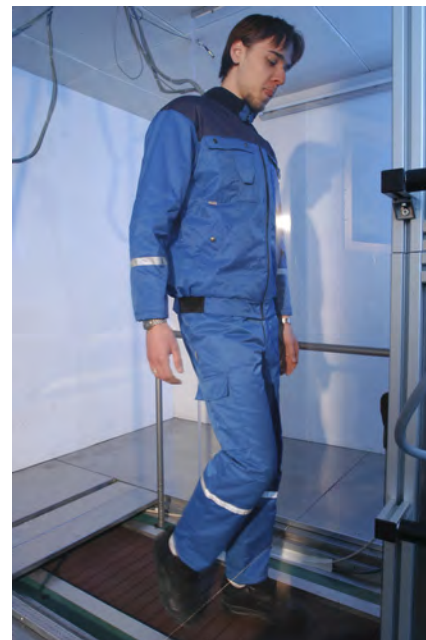
Figure 6: Wearing trials in climatic chamber
