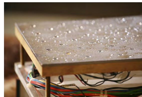
Figure 4: Hohenstein Skin Model (according to EN 31092 / ISO 11092) in sweating mode
