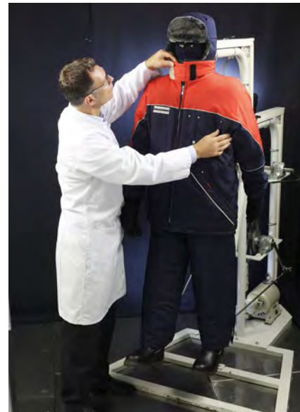
Figure 5: Hohenstein Thermal Manikin "Charlie" (according to ISO 15831 )
