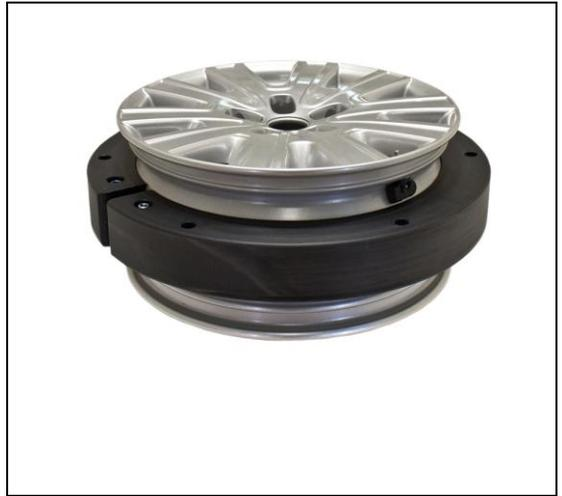
All TSS Heavy Duty Wheels can be delivered as assembly: balanced and complete with Runflat and optional programmable TPMS-sensors.
