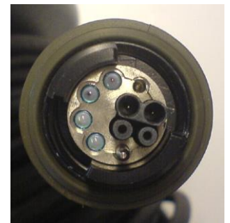
Hybrid Connector for optical- and power connection
