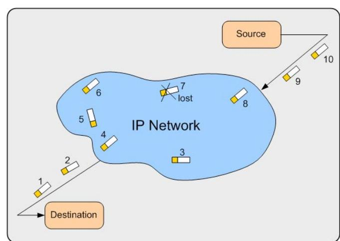
A source sends packets to a destination over TCP. The packets will, due to the IP network definition, not appear in the right order, nor will all packets be received initially.
