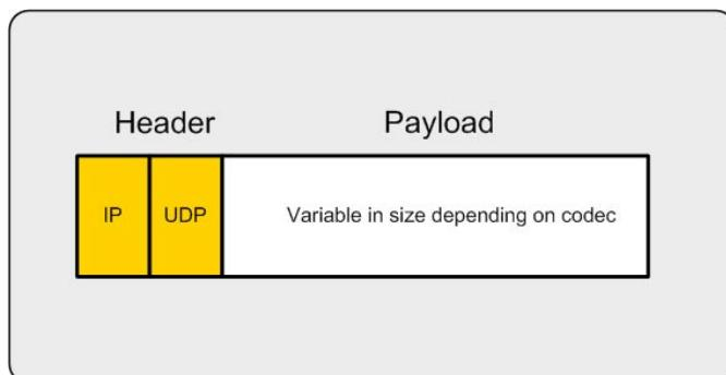
The header contains all the information to identify and address the destination. The payload carries the coded audio samples. At the destination, the incoming packets are stored in a buffer to cope with variations in the packet transport delay. After decoding the incoming data and reconverting it to an analog signal by using a DAC (digital-analog-converter), the signal can be sent to a speaker.
