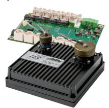
The standard input power requirement of the  $\mu$ MAGBES is 5-36VDC and the device uses less than 6W at full speed with 10 ports operational. Other input voltages can certainly be offered depending on specification. The switch can be operated in an environment of -20°C up to +60°C, and optionally -40°C to +85°C and does not need to be cooled by a fan.
