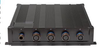
The MIL-PIP46-C12 comes with interfaces like 3x DVI-D, 4x USB 2.0, Audio, dual LAN, and a wide power input. Additional expansions can be done over the internal expansion interfaces such as mPCle, m.2, or PCle/104, These expansions can be done easy and quickly be integrated into the system. This makes the solution flexible and cost efficient customizable.
