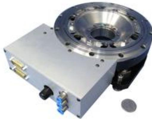
The ZVR vertical platform has a wide, 3-point base with a stepper-motor-driven 10 mm Z-stage. The integrated stainless steel rotation stage features smooth operation utilizing stainless steel ball bearings. It is available in two models, the ZVR-PP with a stepper motor or the ZVR-PC with a servo-driven DC motor. Both rotation stages provide continuous 360-degree rotation for angular travel. An optional linear encoder for the Z-stage or the Z-stage without the rotation stage, are also available.
